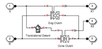
The model implements Dog Clutch, Translational Detent and a modified version of Cone Clutch blocks. Refer to each block reference page for more information on the corresponding block function. You can use a similar approach to model customized versions of the synchronizer. One example is the Gearbox (Detailed) subsystem in the model sdl manual transmission.
