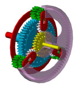
The block models the Ravigneaux gear as a structural component based on Sun-Planet, Planet-Planet, and Ring-Planet SimDriveline blocks. The figure shows the block diagram of this structural component.
