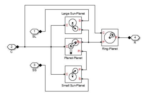
To increase the fidelity of the gear model, you can specify properties such as gear inertia, meshing losses, and viscous losses. By default, gear inertia and viscous losses are assumed negligible. The block enables you to specify the inertias of the internal planet gears only. To model the inertias of the carrier, large sun, small sun, and ring gears, connect Simscape Inertia blocks to ports C, SL, SS, and R.
