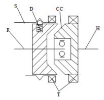
The schematic illustrates a synchronizer in the disengaged state. In this state, the ring (R) and hub (H) shafts can spin independently at different speeds. To synchronize ring
