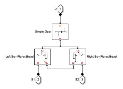
To increase the fidelity of the gear model, you can specify properties such as gear inertia, meshing losses, and viscous losses. By default, gear inertia and viscous losses are assumed negligible. The block enables you to specify the inertias of the gear carrier and internal planet gears only. To model the inertias of the outer gears, connect Simscape Inertia blocks to ports D, S1, and S2.
