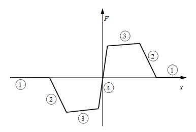
Because the ball is spherical and the notch is symmetric, the horizontal force versus displacement function is symmetric about the origin. (See "Peak Force and Notch Width" on page 1-342.)
